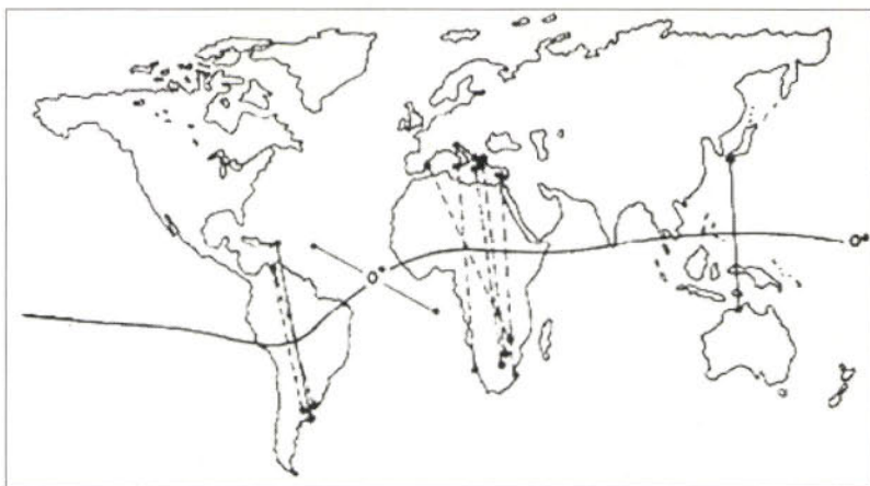
Fig. 1: World map showing the geomagnetic equator and some v.h.f. paths worked via trans-equatorial propagation (see text).
