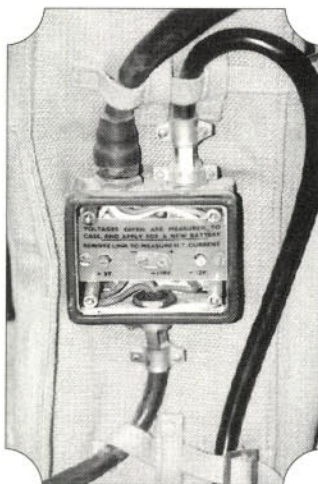
Fig. 3: Testing facilities are provided inside the 46 set junction box (see text).
